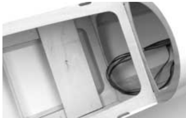
The battery tray is rear mounted for the Zenoah GT-80 or other twin engines.
