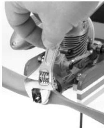
Securely tighten the prop nut using an adjustable wrench.
