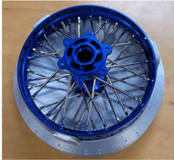
Figure 7. Rear lace fixture with all spokes laced
