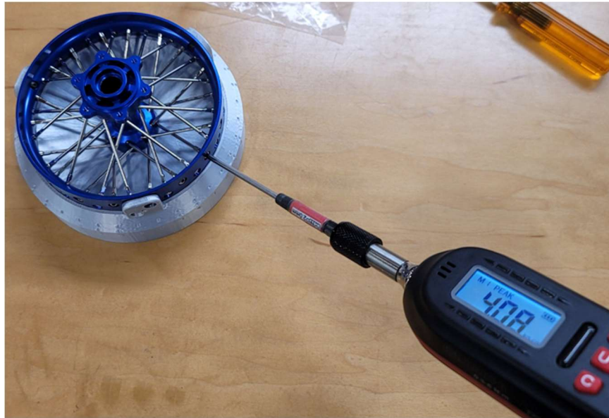
Figure 9. Final torque being applied to spokes
