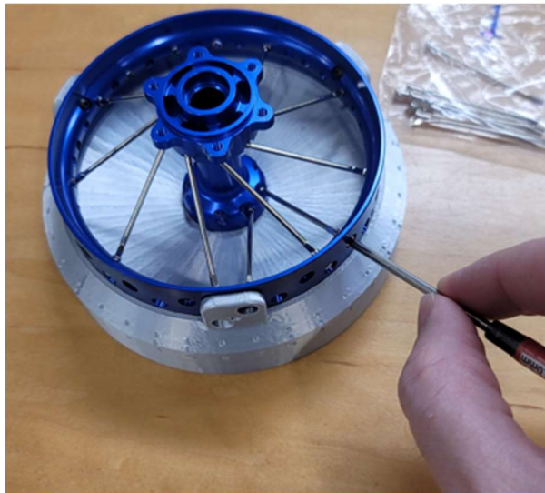
Figure 6. Rear lace fixture with all '1' spokes installed and the 2nd '2' spoke being installed
