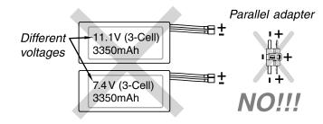
NEVER connect battery packs with different Voltages in Parallel–only combine in Series. Otherwise, the batteries will try to "equalize" with the larger one trying to "charge" the smaller one, thus causing heat and likely a fire.
