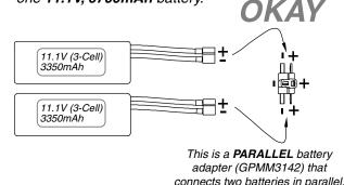
**2)** Connecting batteries in "Parallel" means to connect the +'s to the +'s and the -'s to the -'s. This combines the batteries' capacities, but the voltage remains the same.
