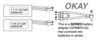
1) Connecting batteries in "Series" means to connect the +'s to the -'s and the -'s to the +'s. This combines the batteries' voltages, but the capacity remains the same.
