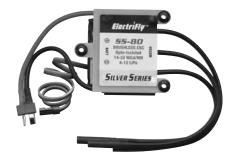
An ESC is basically the device that controls your motor through your radio system. Never run any RimFire motors with a brushed ESC. It will not work and you may damage both the motor and the ESC. Always use a brushless ESC. ElectriFly offers the **Silver Series SS-80 Brushless ESC (GPMM1860)** or the **Silver Series SS-100 Brushless ESC (GPMM1870)** that work well with the RimFire 1.60 (63-62-250) motor.
