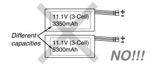
Also NEVER connect battery packs with different capacities in Series or in Parallel.
