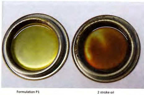
Fig 16 Thermal Stability Formulation P1 compared with 2 stroke oil
