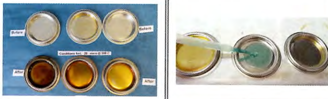
Fig 16 Thermal Stability Formulation P1 compared with 2 stroke oil
